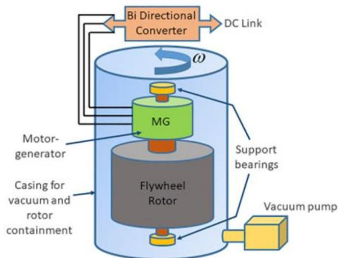
Figure 11: The principle of a Flywheel Energy Storage mechanism<sup>27</sup>
