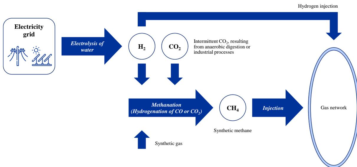
Figure 12: The principle of a Power-to-Gas mechanism<sup>28</sup>
