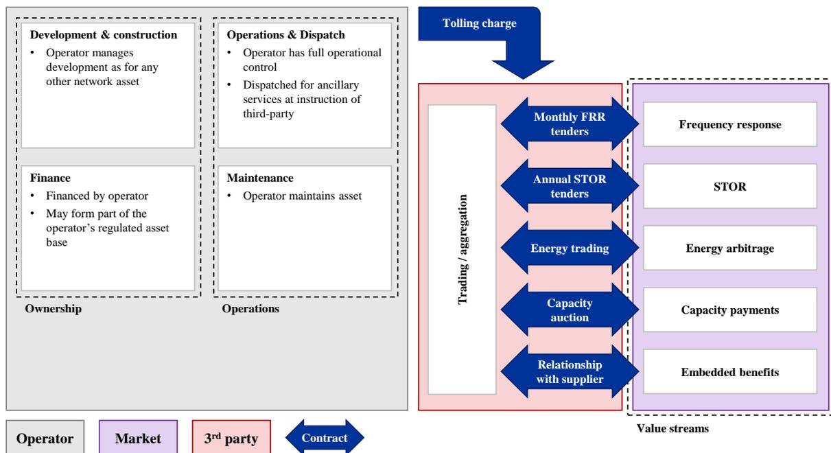
Figure 16: Overview of the Distribution System Operator model<sup>38</sup>
