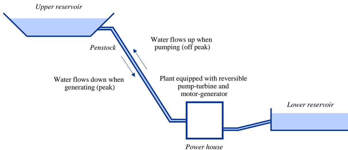
Figure 8: The principle of a pumped storage mechanism<sup>21</sup>
