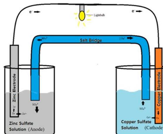
Figure 23: A typical cell used in batteries
