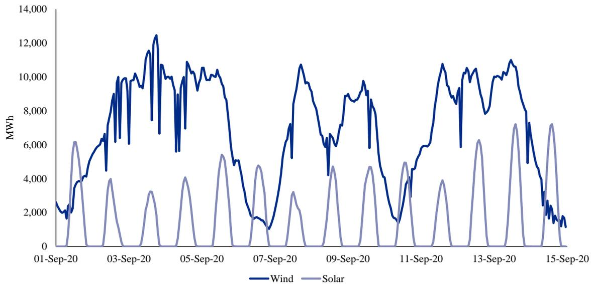
Figure 2: Electricity generation from wind and solar sources in the United Kingdom, between September 1, 2020 and September 15, 2020<sup>4</sup>
