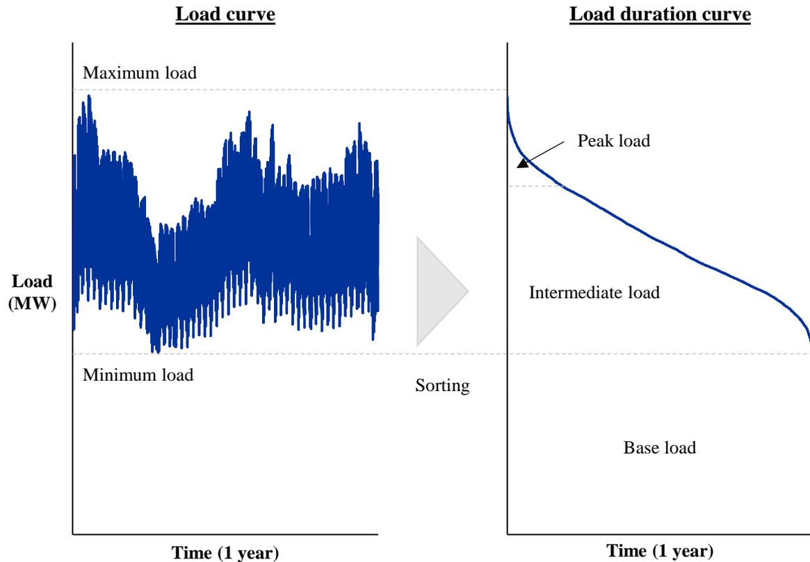
Figure 31: Load and load duration curves for Germany in 2020<sup>53</sup>
