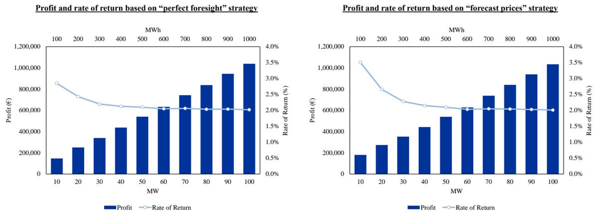
Figure 52: Profit and RoR of Lithium-ion LFP batteries, based on historical and forecast prices, by power and capacity, in France, in 2020
