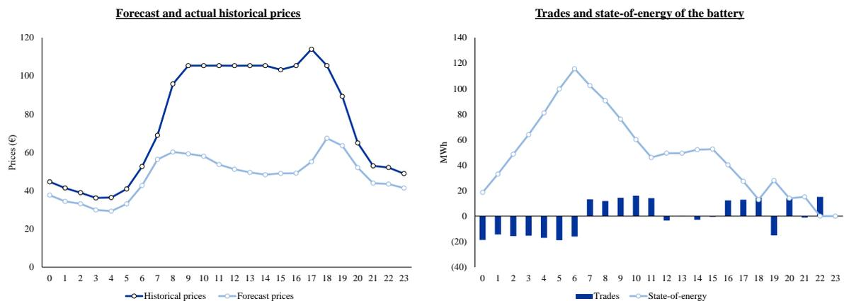
Figure 53: Prices, trades and state-of-energy of the lithium-ion LFP battery on December 9, 2020 (30 MW, 300 MWh)
