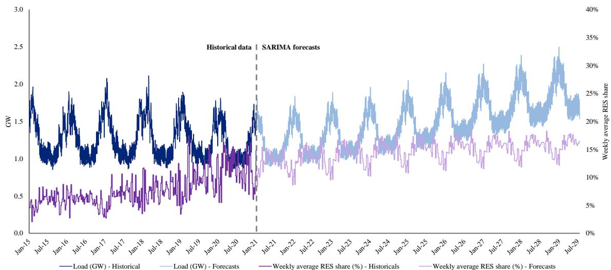
Figure 55:  $SARIMA(1,0,1)(0,1,1)52$  forecasts for load and weekly average RES share in France, between January 2021 and July 2029, based on 2015-2020 data, considering an increase in load and RES share over time<sup>105</sup>
