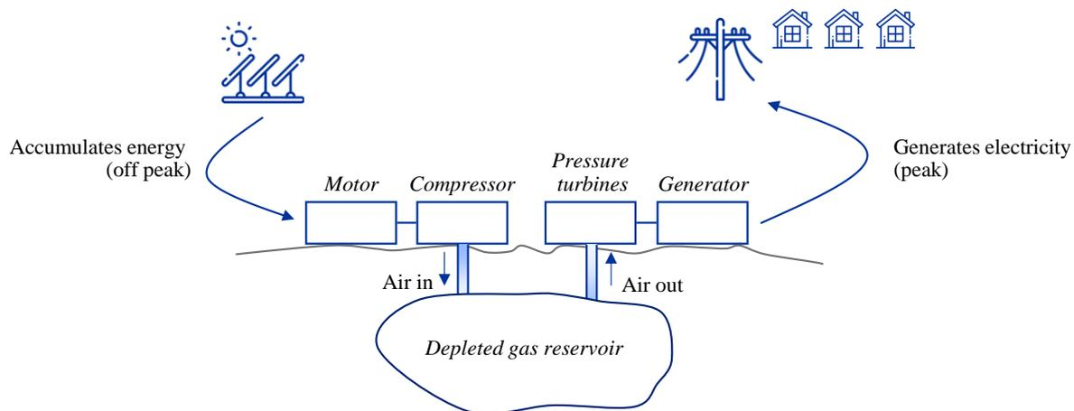
Figure 10: The principle of a Compressed Air Energy Storage mechanism<sup>24</sup>
